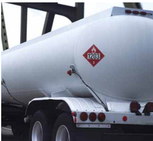
DOT labels posted on vehicles and containers alert people to the dangers of the substances inside.
