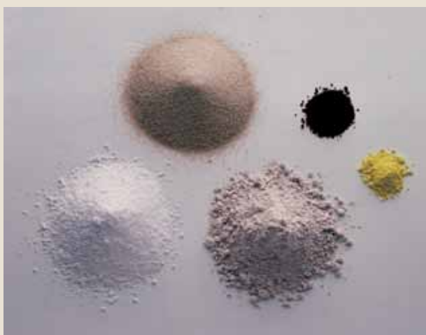
Raw materials of glass: sand, soda ash (sodium carbonate), limestone (calcium carbonate), yellow barium carbonate and brown iron oxide. The last two ingredients are added for color.
