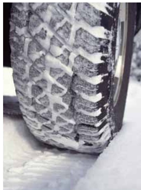
The bobsled and its passengers try to reduce friction. Snow tires increase friction to bring the wheels to a stop.
